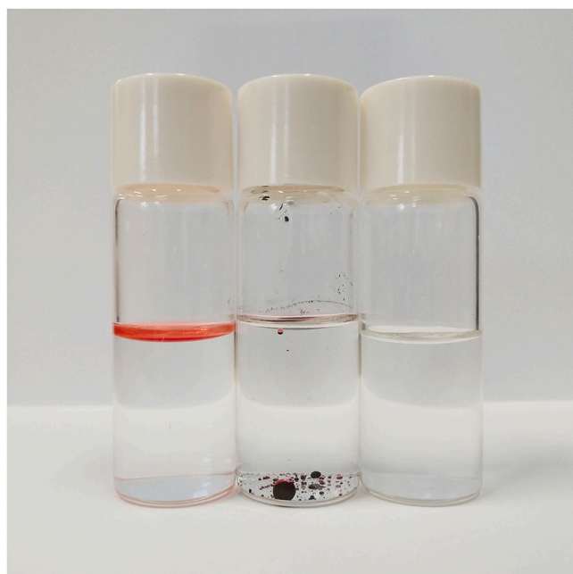
Fig. 8. Oil/water separation involving three stages: left, the water and oil (red) phases; middle, the addition of the minimum quantity of superhydrophobic CuFeCo powder that leads to the formation of an oil-containing marble; and right, pure water without oil.
