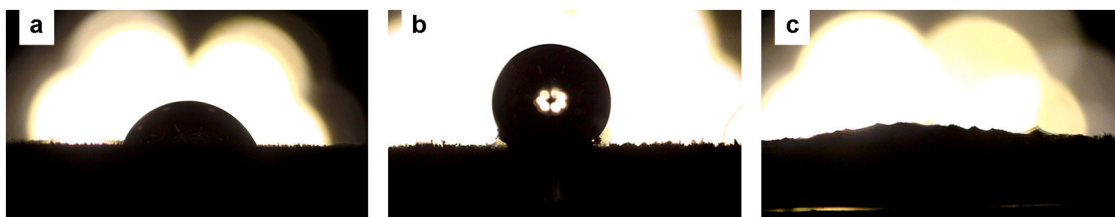
Fig. 7. Images of contact angles measurements: (a) before modification, the surface exhibited a WCA of 87 \pm 1^\circ ; (b) after modification with dodecanoic acid, the WCA was 162 \pm 1^\circ and (c) total adsorption of oil produces an OCA \sim 0^\circ .
