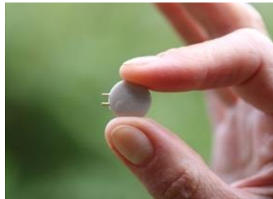
Figure 8. Invilog Research Ltd. implantable nerve stimulator for mice and rats.
