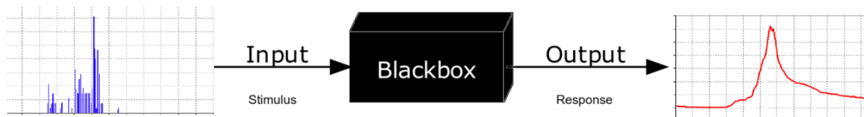
Figure 6: Example of a black box system transforming some discrete data (blue) to continuous (red).
