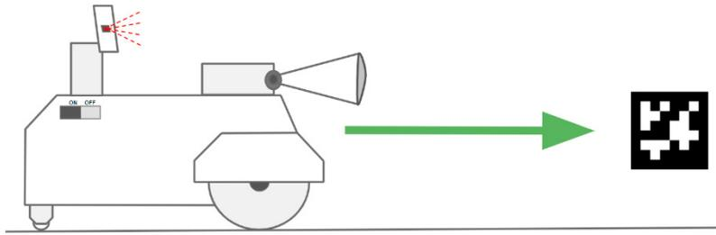
Fig. 5. Experimental set up for testing homeostatic control. Different fiducials are presented to the robot. Only when homeostatic systems are unbalanced, they trigger approach behaviour to the corresponding stimuli.
