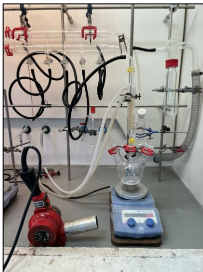
Figure 23. Initial setup for the triallylborane synthesis
