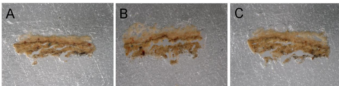
Figure 1.4. Different slices of 20 \mu\text{m} thick of a sample embedded in paraffin. Knife angle changes from 10°(A) to 5°(B) and 0°(C).
