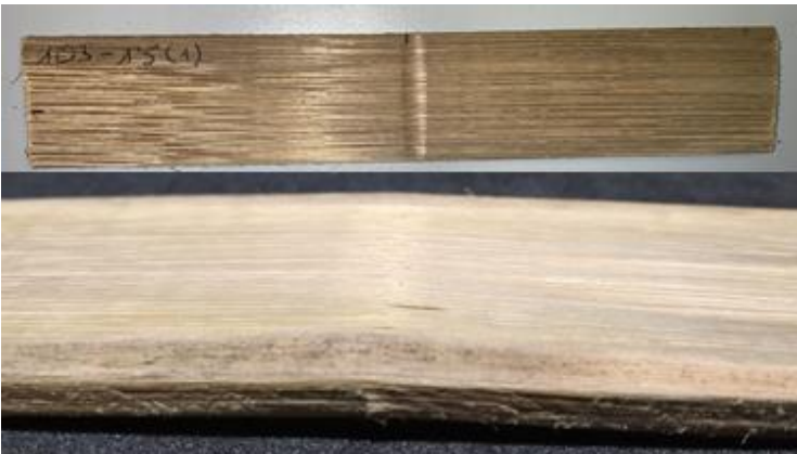
Figure 12. Bamboo test samples after the static three-point bending test.
