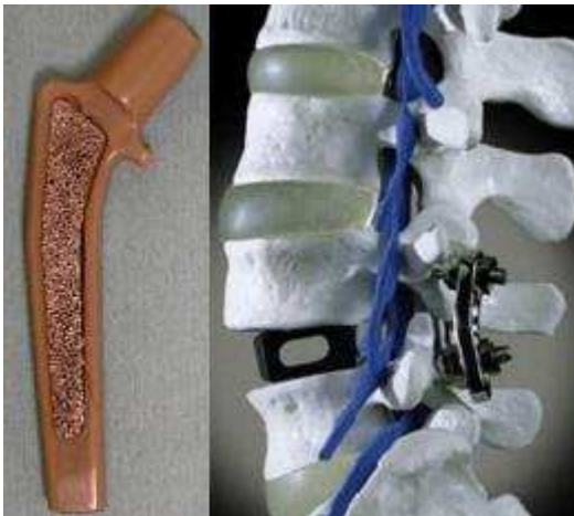
Figure 5. Example of canine hip stems (left) and CFR-PEEK lumbar fusion cage used in concert with posterior screws and rods (right)
