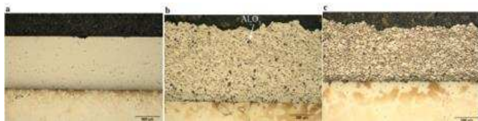
Figure 20. Results of LP-CGS at different mixtures (a) 6061Al coating on AZ91, (b) 6061Al-25% \text{Al}_2\text{O}_3 coating on AZ91 (c) 6061Al-75% \text{Al}_2\text{O}_3 coating on AZ91
