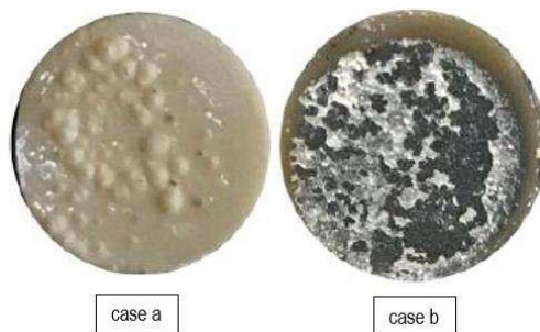
Figure 14. Comparison of the adherence between HA/PEEK and HA/TiO 2 /PEEK
