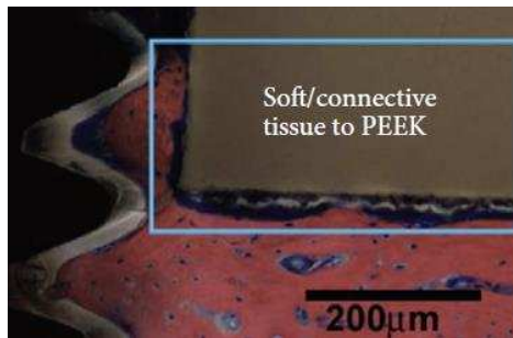
Figure 6. Growth of soft/connective tissue around PEEK
