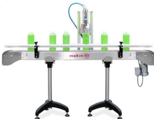
Figure E5. SERIE ERS cap packaging equipment, EQUITEK.
