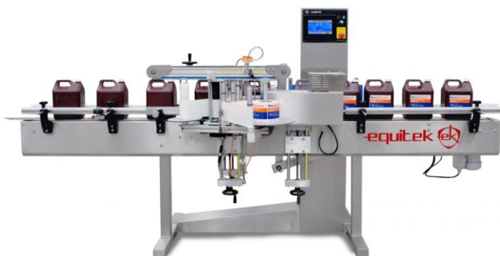
Figure E6. SERIE ESZ bottle labelling equipment, EQUITEK.
