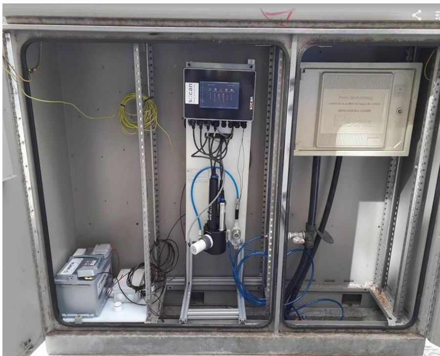
Figure 9: Installation of Nano station on Dr. Trueta. This facility is inside a sampling cabinet owned by Aigües de Barcelona
