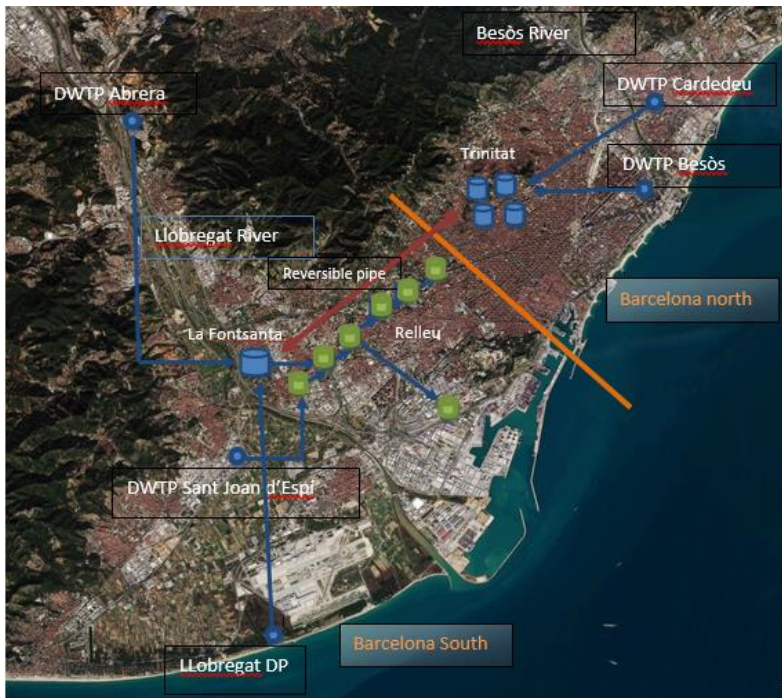
Figure 2: Map of Barcelona city showing the sources of supply, main pipelines and reservoirs.
