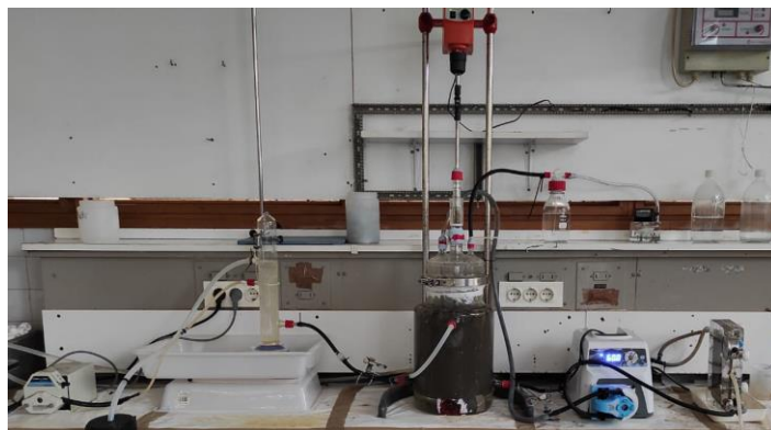
Figure 2.1. Lab-scale AnMBR set-up used in Publication II.
