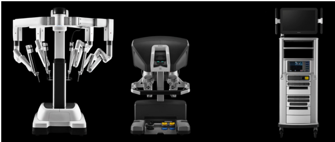
Figure 2. Da Vinci components: Surgical Cart, Surgical Console and Vision Tower [13].
