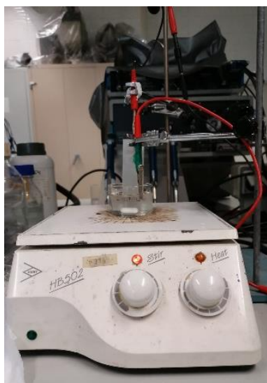
Figure 10 Magnetic stirrer with anodizing equipment set-up.
