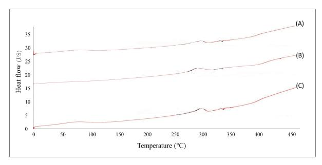
**Figure 1.** DSC thermograms of tizanidine with physical mixtures of chitosan and thiolated chitosan (A), EC and PVP (B), and Eudragit RL100 and PVP (C).
