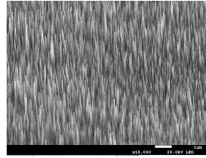
FIG. 2: FE-SEM image of MWCNTs before ammonia plasma treatment.
