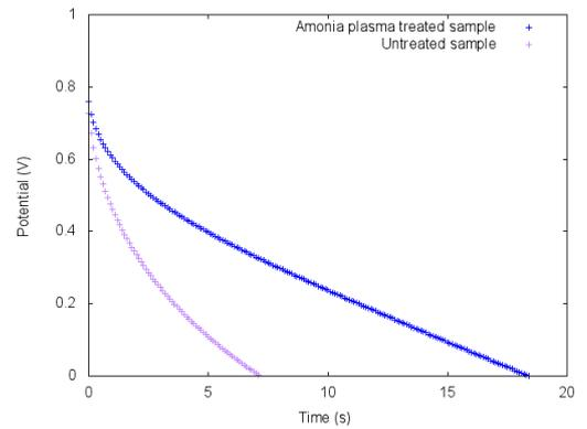
FIG. 5: Comparison between a discharge curve from a charge - discharge experiment involving ammonia plasma treated and non-treated samples MWCNTs with a current set to 500  $\mu\text{A}$ .
