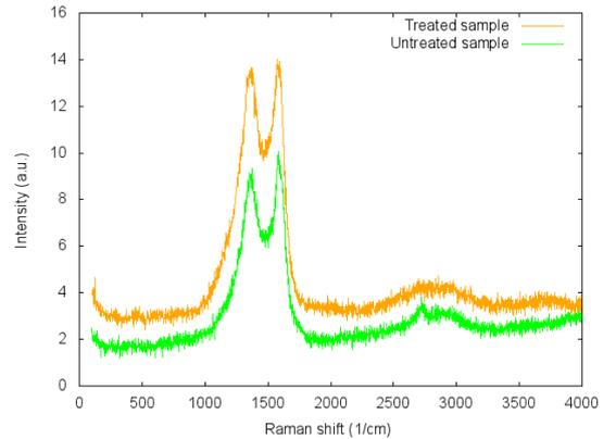
FIG. 3: Raman spectra of untreated and NH<sub>3</sub> plasma treated CNTs samples. In the untreated sample, the D band, the G band and the R ratio had the following values: 1369 cm<sup>-1</sup>, 1581 cm<sup>-1</sup> and 0.911. On the other hand, in the treated sample, the D band, the G band and the R ratio had the following values: 1363 cm<sup>-1</sup>, 1576 cm<sup>-1</sup> and 0.983.
