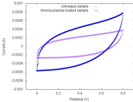
FIG. 4: Cyclic voltammograms of ammonia plasma treated and non-treated samples MWCNTs at a scan rate of 50 mV/s in a 0.1 M  $\text{Na}_2\text{SO}_4$  solution
