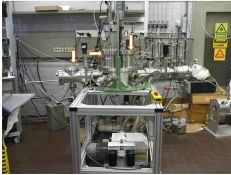
FIG. 1: Picture of the PECVD reactor used to create the CNTs involved in this study. The arrows show, from left to right: the place to introduce the sample inside the closed compartment and three different heads; one for iron sputtering, one for silicon sputtering and one for heater and PECVD reaction. [9]
