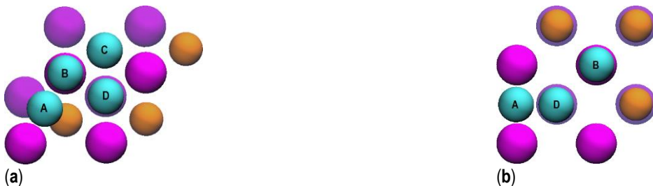
Figure 2. Possible adsorption sites for ^*H . (a) (111) facet of an fcc metal. (b) (100) facet. A) bridge, B) top, C) FCC hollow and D) HCP hollow. Purple atom: Pt, blue atom: H, orange atom: Cu in the subsurface.
