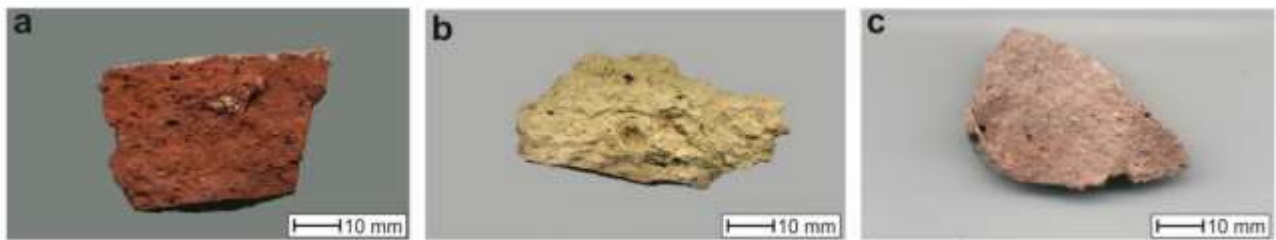
Figure 2 An example of macro photos under reflected light of the bricks of Hagia Sophia representative of the qualitative chromatic features. a) Sample BAS3; b) Sample BAS7; c) Sample BAS28.
