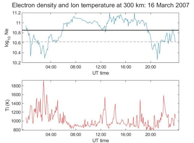
FIG. 1: Main ionospheric parameters as a function of UT time at an altitude of 300 km. On top: Electron density. At the bottom: Ion temperature. The wide black line represents the daily mean of the electron density, while the narrow dashed line represents the same mean minus a standard deviation.
