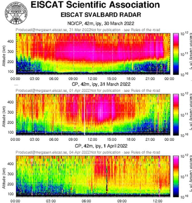
FIG. 2: Electron density profiles taken during the experiment at the EISCAT Svalbard radar. From top to bottom: 30 of March (whole day), 31 of March (whole day), 1 of April (half the day).
