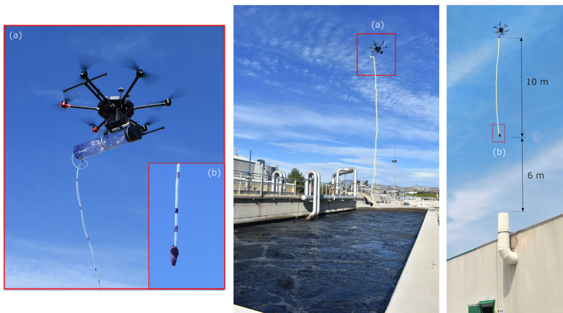
Fig. 4. Photos of the drone during sampling of the bioreactor at 1 m distance (center picture) and the deodorisation chimney at 6 m distance (right picture). The height of the drone in these two examples was 13 m a.g.l. and 25 m a.g.l., respectively. The left picture shows close-up views of (a) the drone and payload and (b) the inlet of the weighted sampling tube.
