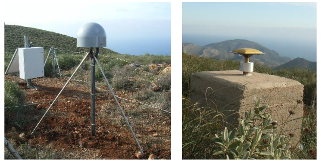
FIG. 2: Example of geodetic monuments used in the study located at Cabo de Gata (Almeria). A: cGPS permanent station; B: sGPS monument with an antenna at RELL of the CuaTeNeo network [12].
