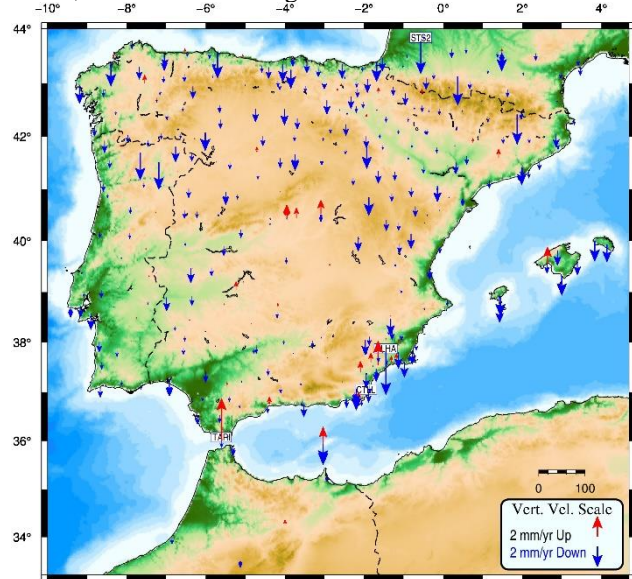
FIG. 6: Vertical velocity field from GPS measurements. The stations with a speed <5 mm/yr are excluded.
