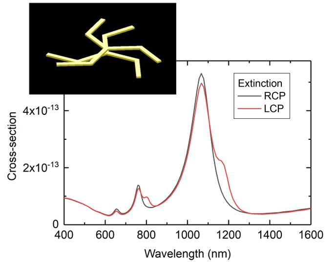
FIG. 3: Two stacked triskelia (inset). The diagram shows the triskelion total extinction as a function of the wavelength for both RCP and LCP light impinging normal to the structure.
