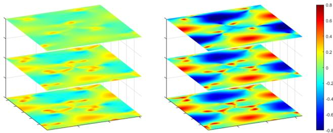
FIG. 6: Local dichroism of the modulus of the electric field computed by Eq. (1) for both  $p = 1235$  nm (left column) and  $p = 1300$  nm (right column) measured for 1074 nm and 1134 nm, respectively, and calculated over three horizontal planes: one 5 nm over the top triskelion (top row), one in the middle (mid row) and one 5 nm over the bottom triskelion (bottom row).
