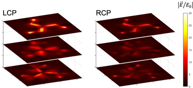
FIG. 4: Distribution of the modulus of the electric field normalised to the modulus of the incident field for 1178 nm RCP (right column) and LCP (left column) light impinging normal to the structure, measured over three horizontal planes: one 5 nm over the top triskelion (top row), one in the middle (mid row) and one 5 nm over the bottom triskelion (bottom row).
