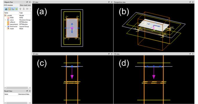
FIG. 7: Lumerical user interface, where views along the planes XY (a), XZ (c) and YZ (d) and a perspective view (b) of the designed structure are shown.
