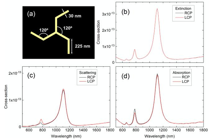
FIG. 1: Top view of the free-standing triskelion (a). Diagrams (b), (c) and (d) show, respectively, the extinction, the scattering and the absorption as a function of the wavelength for both RCP and LCP light impinging normal to the structure.
