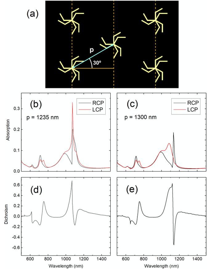
FIG. 5: Hexagonal lattice of triskelion stacks (a), where  $p$  is shown and equivalent lines of points of the Bravais lattice are represented as vertical dashed lines. Diagrams (b) and (c) show the absorption for both RCP and LCP light impinging normal to the structure for  $p = 1235$  nm and  $p = 1300$  nm, respectively. The corresponding dichroism computed through Eq. (1) is shown in diagrams (d) and (e).
