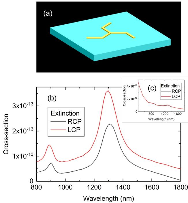
FIG. 2: Triskelion structure over a 200 nm silica ( $\text{SiO}_2$ ) layer (a). Diagrams (b) and (c) show the triskelion effective  $E$  and total  $E$ , respectively, as a function of the wavelength for both RCP and LCP light impinging normal to the structure.
