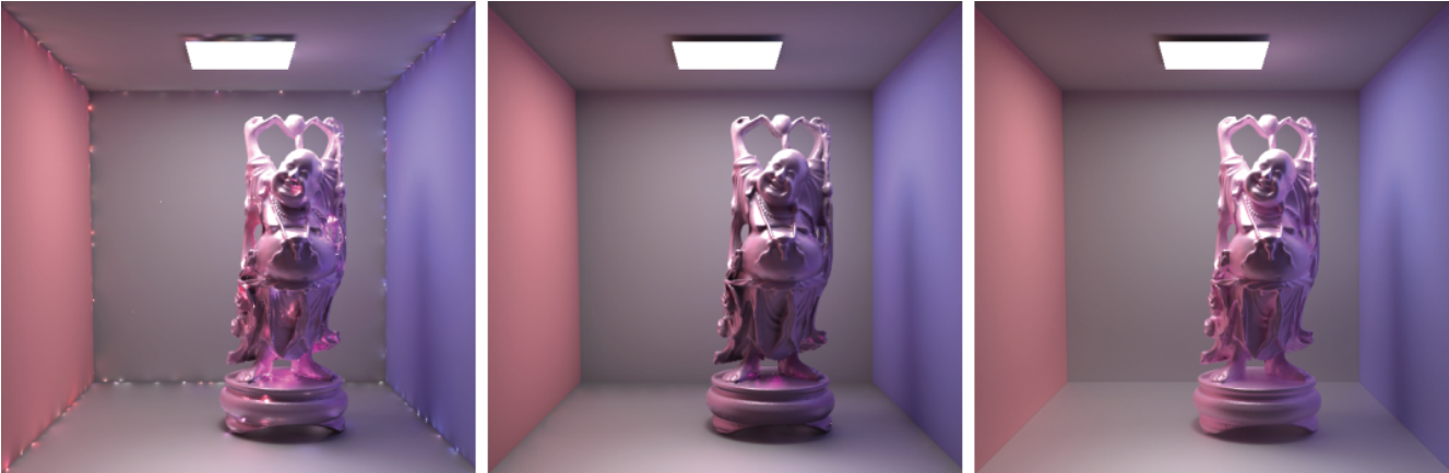
Figure 2.3.2 Illustration of singularities. From left to right: Unbounded VPLs, Bounded VPLs, unbiased solution (non-VPL) (Source: [6])
