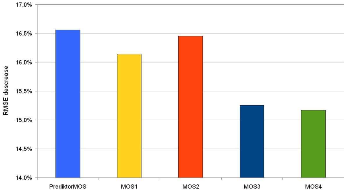
Figure 11a – Mean improvements of different MOS types in respect to NWP forecast in Klim wind farm
