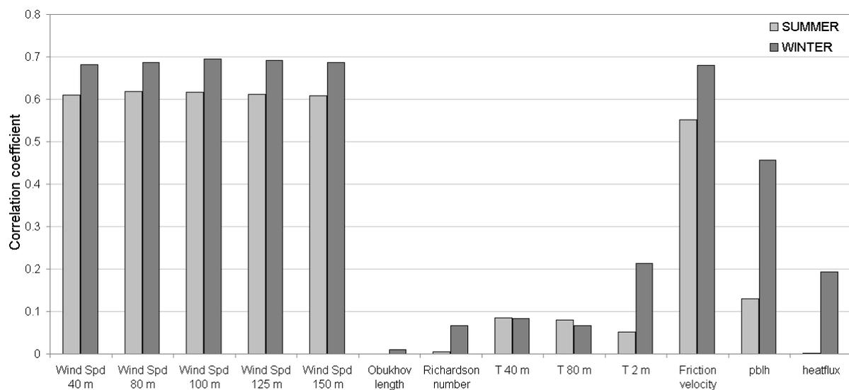
Figure 8b – Correlation coefficient for cycle 1 of the predictors' selection for a summer (August) and a winter (January) stratified MOS in Golagh wind farm
