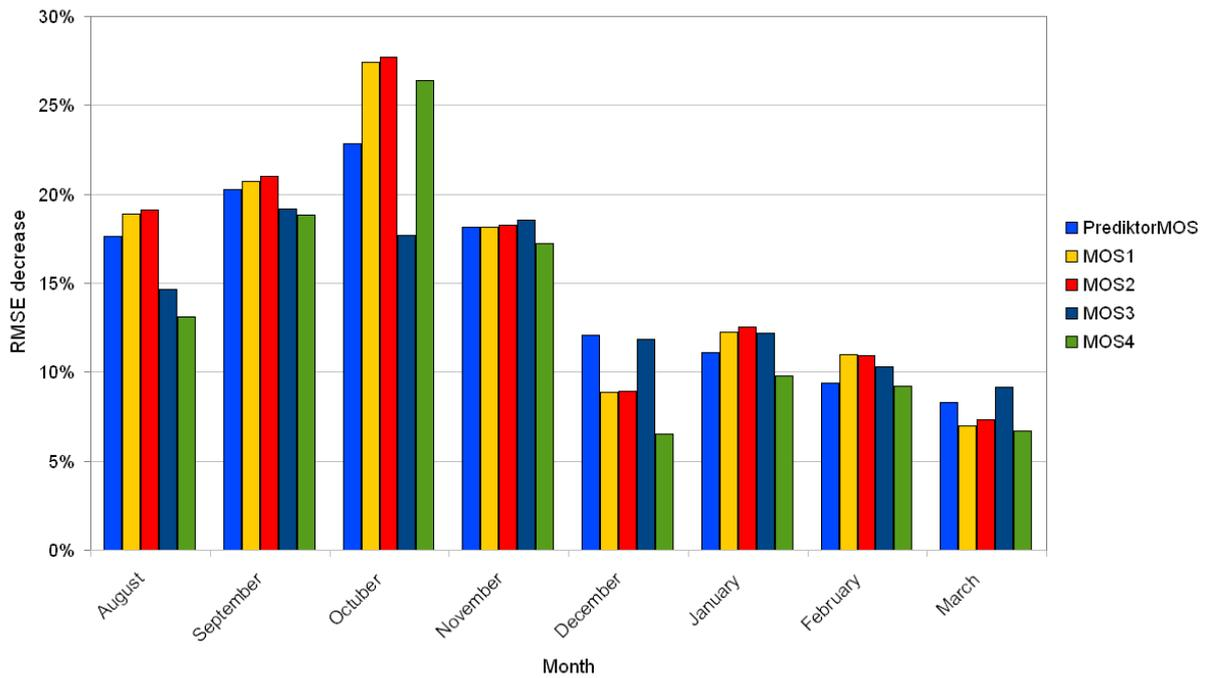
Figure 10b –Improvements in respect to NWP forecast with different MOS types (monthly stratified MOS) in Golagh wind farm
