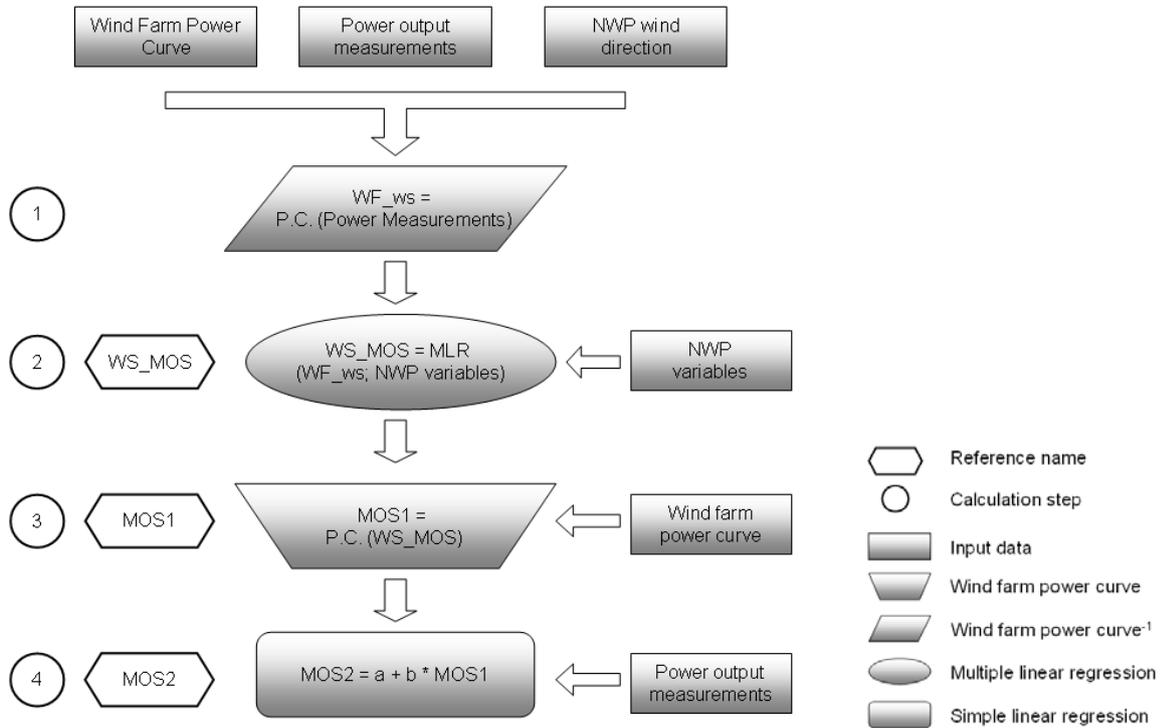
Figure 2 – Diagram chart of the proposed MOS method. Shapes on the bottom right indicate the type of calculation or method implemented at each step: wind farm power curve, multilinear and linear regression
