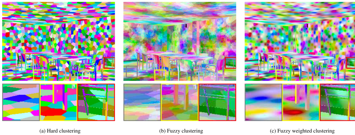
Fig. 4. Visualization of the different tested clustering techniques when clustering the shading points (3D spatial clustering). Note that the border between neighboring clusters is progressively faded from left to right. The corresponding rendering results are shown in Fig. 5.
