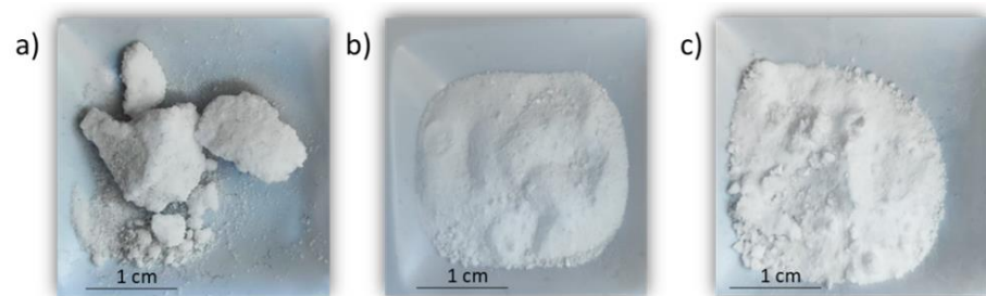
Figure 8. Effect of moisture on physical properties (water absorption) of (a) pure NaNO 3 , (b) NaNO 3 /SiO 2 NPs (1% wt.) and (c) NaNO 3 /Al 2 O 3 NPs (1% wt.).
