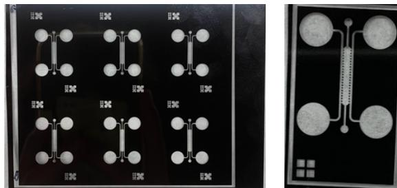
*The main chamber (simulating the brain) can be distinguished, connected through little openings to the blood vessel chambers. The circles correspond to the holes from where the cells will be introduced into the device. Source: myself, in IBEC lab*
