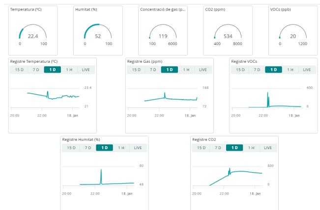
FIG. 7: Dashboard of our device. Real-time values are shown in gauges with a historic of the last 24 hours.
