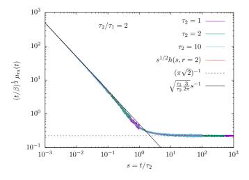
FIG. 8. Scaling plot of the mean-crossing intensity for  $\tau_2/\tau_1 = 2$ . The noisy colored lines correspond to the simulation results for different values of  $\tau_2$ . The curved (red) solid line corresponds to the analytical result in Eq. (68). The straight solid and dashed (black) lines correspond, respectively, to the short-time and long-time asymptotic regimes in Eq. (71).
