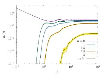
FIG. 14. Total crossing intensity  $\mu_u(t)$  for the damped oscillator with  $\beta = 0.1$ , k = 1,  $\omega_0 = 1$ ,  $x_0 = 0$ ,  $y_0 = 0$ , and dt = 0.01, for different levels u. The noisy colored lines show the simulations results averaged over  $10^6$  trajectories (labels for different u are, from top to bottom, in the same order as the lines). The smooth (black) curves are the analytical results, obtained substituting Eqs. (82), (83), (84), and (85) into Eq. (26).
