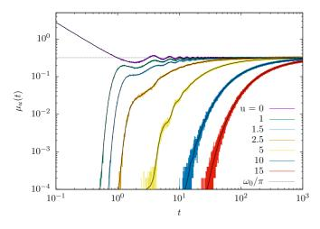
FIG. 15. Total crossing intensity  $\mu_u(t)$  for the undamped oscillator ( $\beta = 0$ ) with k = 1,  $\omega_0 = 1$ ,  $x_0 = 0$ ,  $y_0 = 0$ , and dt = 0.01, for different levels *u*. The colored lines show the simulations results averaged over 10<sup>6</sup> trajectories (labels for different *u* are, from top to bottom, in the same order as the lines). The smooth (black) curves are the analytical results, obtained substituting Eqs. (98), (99), and (100) into Eq. (26).
