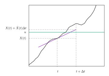
FIG. 1. Illustration of an upcrossing event. The irregular (black) line represents a simulated random trajectory X(t), the straight oblique (purple) line has slope  $\dot{X}(t)$ . If  $\Delta t$  is small enough, then X(t) will cross the level *u*, represented by the horizontal solid (green) line in the interval  $(t, t + \Delta t)$  if  $\dot{X}(t) > 0$  and  $u - \dot{X}(t)\Delta t \leq X(t) \leq u$ .
