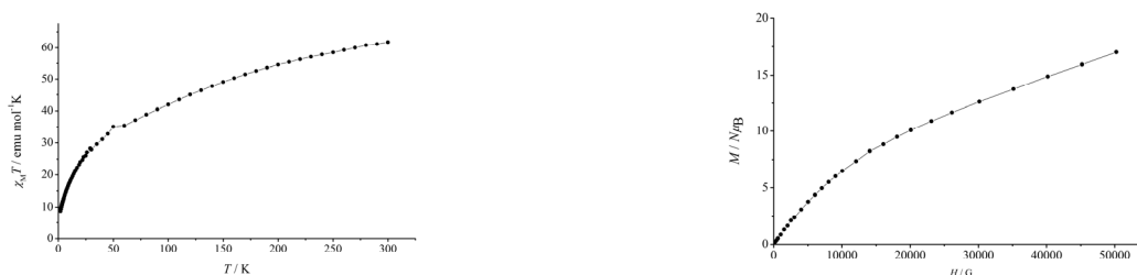
Figure 5. Magnetic data for complex 2 , showing a \chi T vs. T plot collected at 5000 G and magnetization vs. field plot at 2 K.
