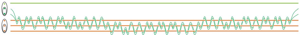
Figure 4.4: Full construction of a  $i \cdot \text{CNOT}$  gate, which can be decomposed into the operations of injection,  $i \cdot \text{NOT}$  weave and inverse injection.
