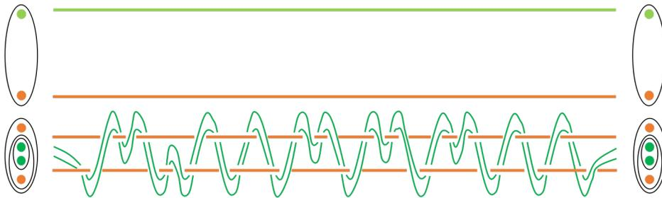
Figure 4.3: Step two of the **CNOT** gate. The control pair is woven within the injected target qubit. An approximate  $i \cdot \text{NOT}$  gate is carried out when the control pair has global charge  $\tau$ .
