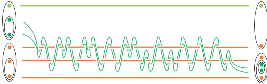
Figure 4.2: Injection weave and step one of the **CNOT** gate. If the control qubit is in the state  $|1\rangle$ , then the global charge of the injected anyons is  $\tau$  and the result is to produce a target qubit with the same charges as the original but with its middle anyon replaced by the control pair.
