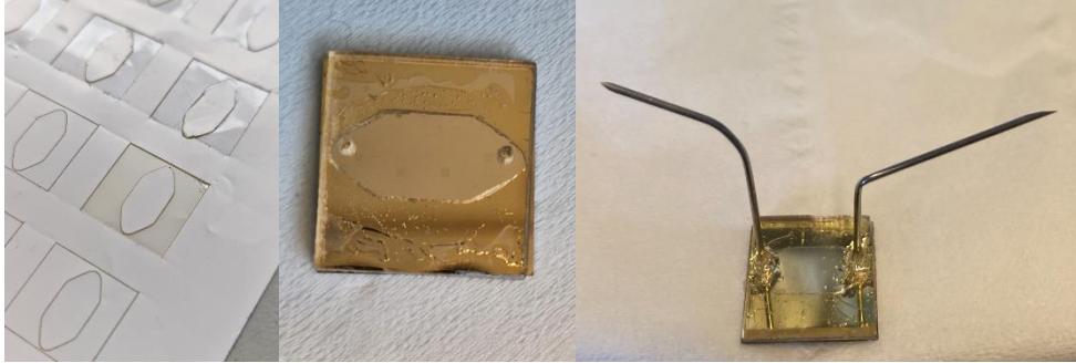
Figure 15: a) microfluidic design on a double-sided adhesive tape b) methacrylate lid incorporated onto the surface of the chip c) inlet and outlet syringe needles placed and sealed with super-glue onto the methacrylate lid.
