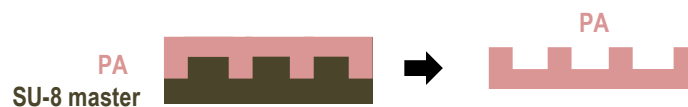
Figure 15: Scheme of PA microchannels obtention from a direct molding of the master.
