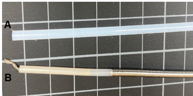
Figure 1 Example of bare core (A) and core with a PTFE liner and braid (B).
