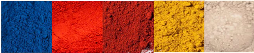
Figure 1. Powder pigments from left to right: Blue CI 42090 (173), Red CI 15850 (174), Red iron oxide CI 77491 (175), Yellow iron oxide CI 77492 (176), Titanium dioxide CI 77891 (177).
