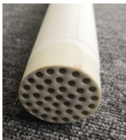
Figure 2. Inorganic membrane composed of zirconia (Made-in-China)
