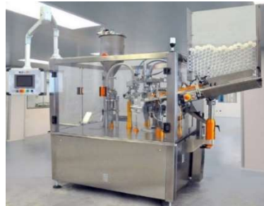
Figure 7: Tube filling and closing Machine from JM Filling Solutions.
