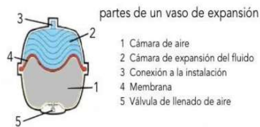
Figure 14 Components of a closed expansion vessel.
