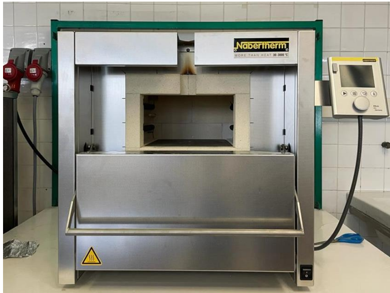
Figure 10. Chamber furnace employed for measuring ash and volatile matter content.
