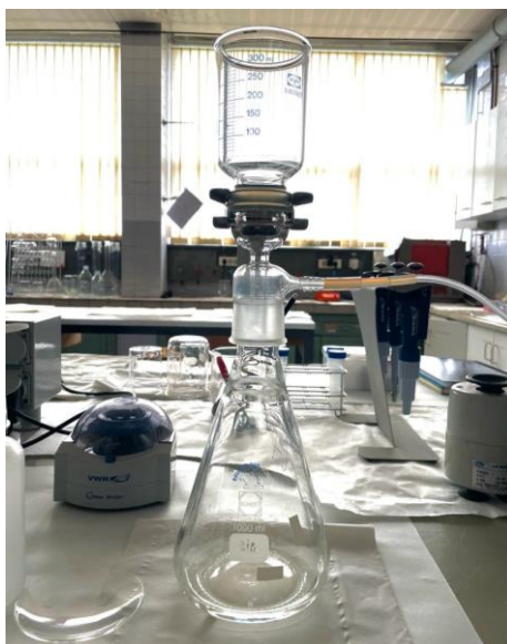
Figure 9. Assembly for total suspended solids determination.
