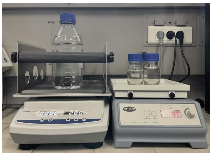
Figure 8. Experimental device for adsorption experiments.
