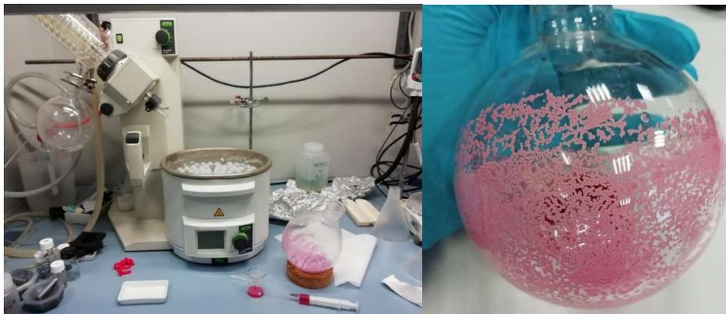
Figure 5: Left: Experimental setup for the synthesis of the catalysts. Right:  $\text{Co}(\text{NO}_3)_2$  Impregnated  $\gamma\text{-Al}_2\text{O}_3$  (before calcination).
