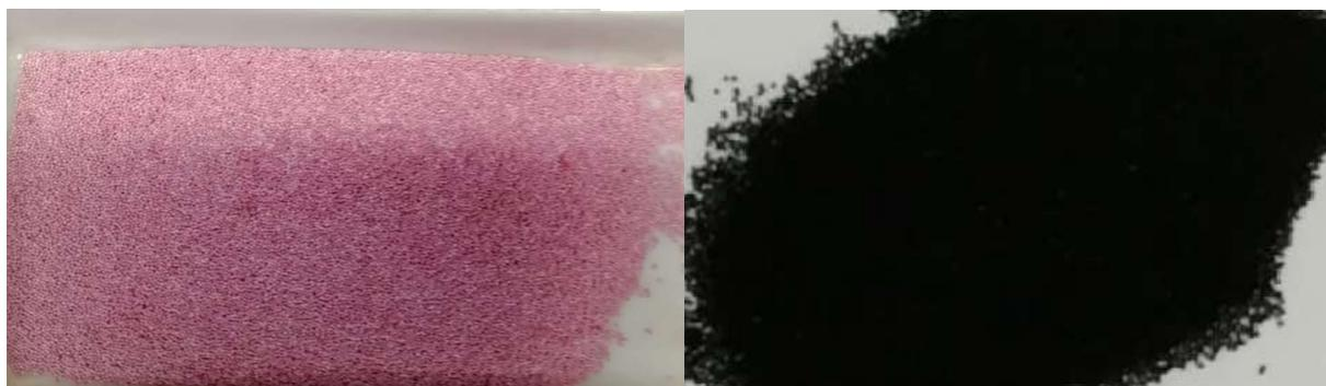
Figure 6: Left: Supported Cobalt Nitrate over  $\gamma$ -Al<sub>2</sub>O<sub>3</sub>, final product after the 2<sup>o</sup> drying. Right: Supported Cobalt oxide over  $\gamma$ -Al<sub>2</sub>O<sub>3</sub> after being calcinated at 500°C
