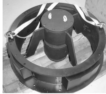
Figure 2. Spider vanes assembly and focus system for the CCD.
