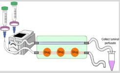
The device consists of 2 cylindrical channels which are fully embedded in gelatin-fibrinogen ECM. In one channel, epithelial cells isolated from kidney organoids are seeded and perfusion is applied through the second channel which mimics basolateral drug uptake.
