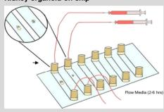
The device has 6 culture channels with an inlet and an outlet each. Kidney organoids grown in static culture are pipetted in these channels which are already covered with Reduced Growth Factor Geltrex and cultured under different fluidic regimes.
