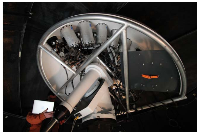
Figure 7. Mathis German Equatorial mount, the tubular base structure, and the mounted mushroom—showing the instrument inset, mass alignment, and camera accessibility.
