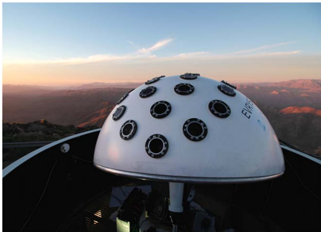
Figure 1. Evryscope, a two-dozen-camera array mounted into a 6-ft diameter hemisphere, deployed at the CTIO observatory.
