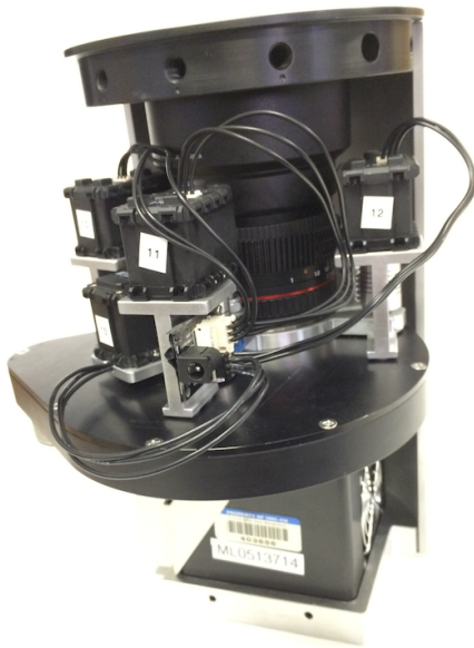
Figure 6. The Robotilter automated tilt removal and focus optimization mechanism. Servo movement adjusts the lens plate relative to the CCD. Exploded views of the servo, flexible shaft coupler (to prevent binding), fine adjustment shaft, and brass insert are shown along with the focus adjustment servo and gear.
