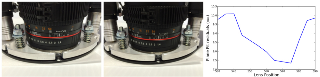
Figure 12. Left: The potential focus range of the lenses. Right: The field flatness as a function of lens focus position (530-590 in servo position for this lens), by computing the residuals of the plane fit to the measured 3-D focal plane contour. The flattest field is at \approx 15 servo steps from the maximum lens focus, on average for the Evryscope camera assemblies.
