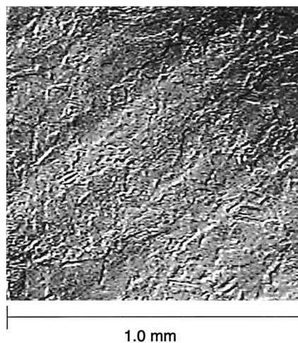
Fig. 8. Nomarski micrograph of the electroplated gold A surface.
