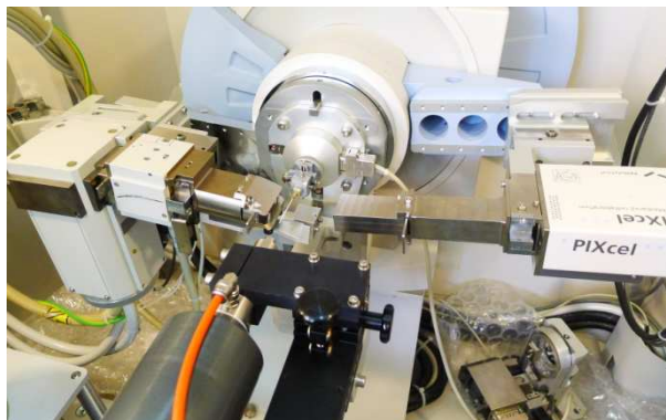
Figure 14: Cu K\alpha_{1+2} configuration with focalizing mirror, capillary stage, low temperature attachment and PIXcel detector in an X-ray powder diffractometer PANalytical X'Pert PRO MPD \theta/\theta at the CCiTUB.
