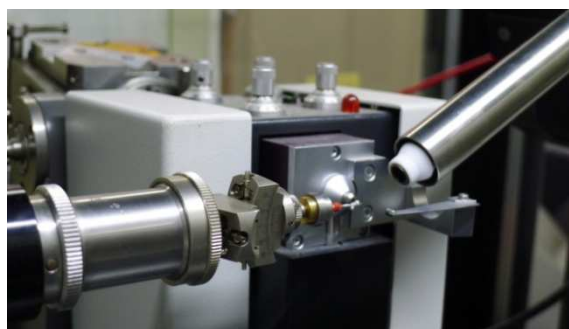
Figure 2: Detail of the goniometer and low temperature system in the MAR345 single crystal diffractometer at the CCiTUB
