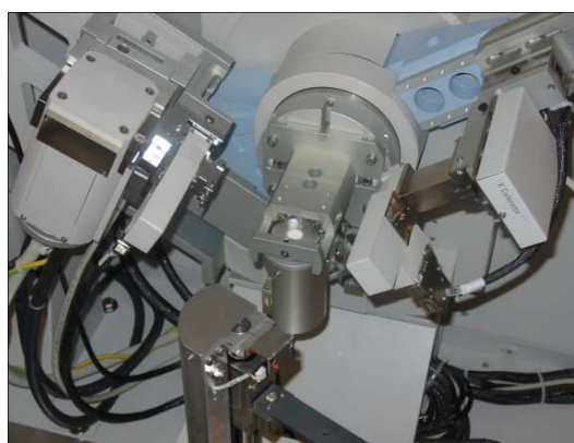
Figure 12: \theta/2\theta goniometer, in Bragg-Brentano Cu K\alpha_{1+2} configuration, of the X-ray powder diffractometer PANalytical X'Pert PRO MPD alpha1 at the CCiTUB.
