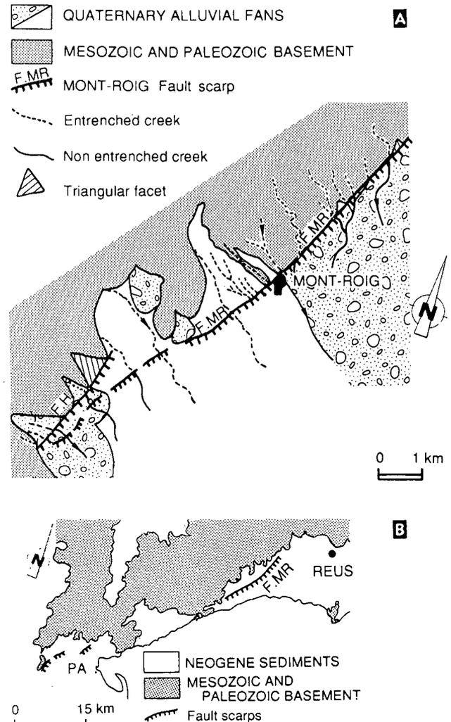
Figure 4. **A.** The Mont-roig scarp cutting through two generations of alluvial fans. The drainage is entrenched in the upthrown block of the fault and it is not in the downthrown block. FH Hospitalet fault. FMR Mont-roig scarp. **B.** Situation of the scarps localized in the studied area. PA, Pla de l'Ampolla.
