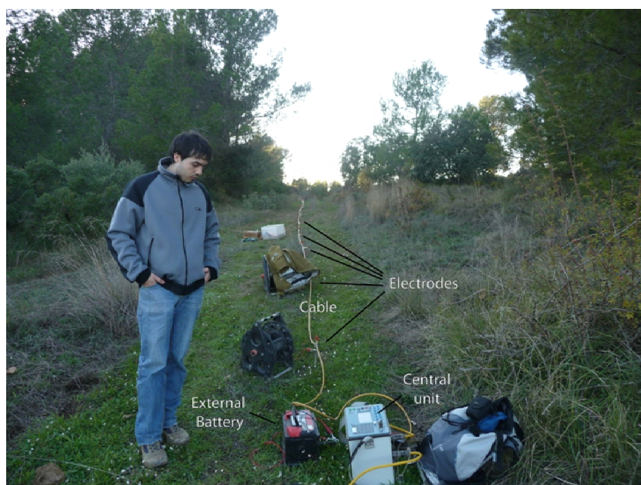
Figure 3.6: Photograph displaying the disposition of an ERT device spreaded in field. The central unit (a Syscal Pro Switch with 48 electrodes is displayed in the photograph) links the two cables with 24 electrodes each. In this case the spacing between electrodes is of 2 meters.
