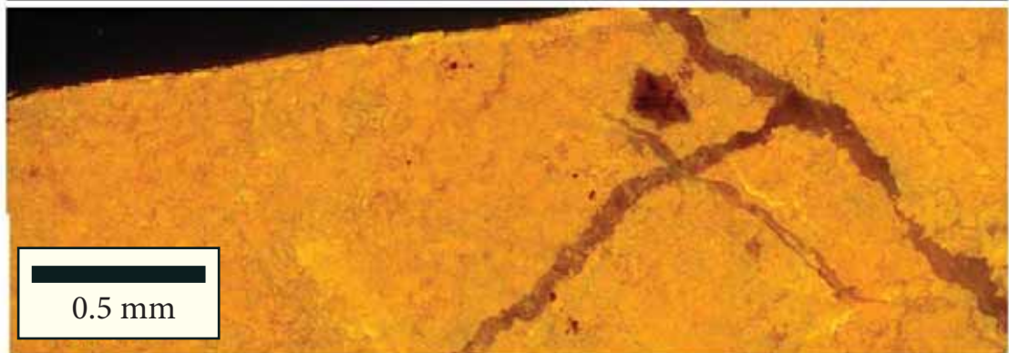
Serie 2. Microfractures cemented with calcite.
