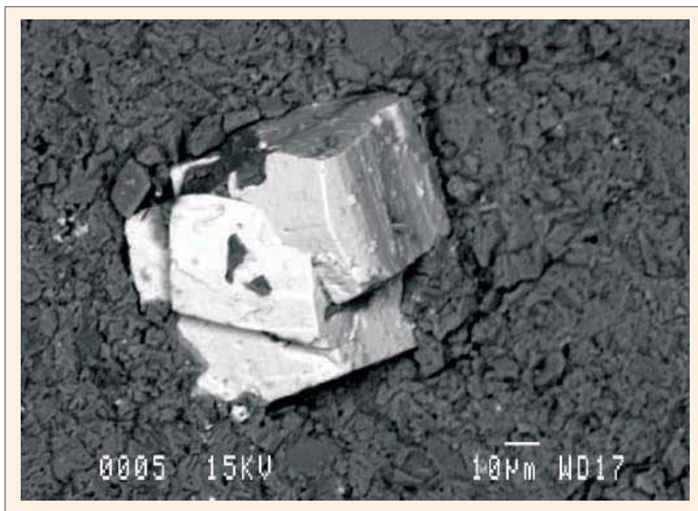
Fig. 6.9. Backscattered image of pyrite pseudomorph. The striated faces are typical of the precursor pyrite.
