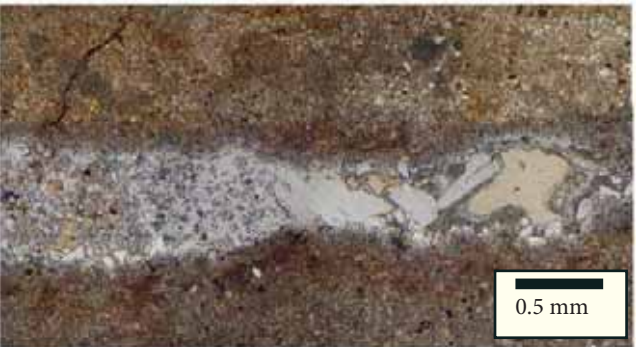
Serie 4. Dedolomite corrosion of Dd1 in a fracture partially sealed with dickite (dk).
