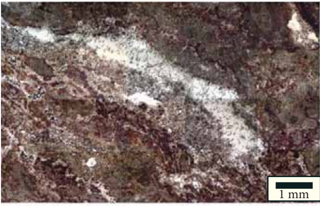
Serie 3. Dedolomite cemented cavity.
