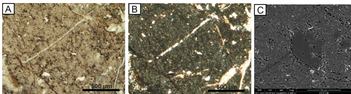
Figure 4.25. Pseudotachylyte microphotographs. A-B) Pseudotachylyte affected by later laumontite and calcite fractures (plane light and cross-polarized light, respectively). C) SEM image of the pseudotachylyte. Observe the fine-grained matrix where micrometric micacrystals have grown by later alteration and the corroded geometry of the quartz clast.
