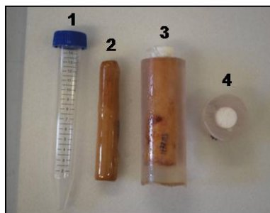
Figure 3-10. Sequence of sample preparation for the permeability test: (1) 15 mL polypropylene tube used as template; (2) resulting polyHIPE after being coated with the first layer of adhesive resin; (3) polyHIPE after coating with epoxy Araldite 2020 ® ; (4) transversal view of the cut sample (25 mm diameter) containing the polyHIPE (15 mm diameter), which is ready for permeability studies.
