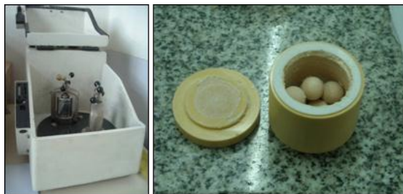
Figure 3-2. Planetary ball-milling (left) used to carry out the solid-state reactions. Picture on the right shows the vial and the milling-balls, both made of \text{ZrO}_2 .
